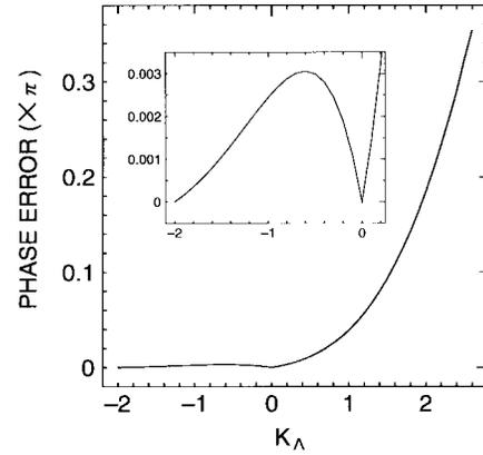
Fig. 4. Maximum phase error versus  $K_\Lambda$  when  $\Lambda = 10$ ,  $\omega_p = 0.4\pi$ ,  $\omega_s = 0.6\pi$ , and  $W(\omega) = 1$ .
