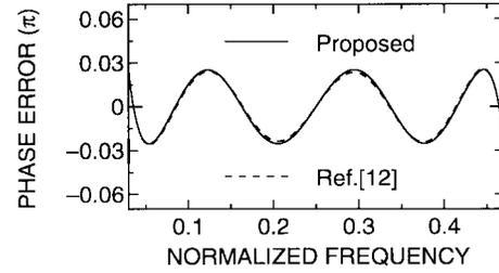
Fig. 3. Phase errors of Hilbert transformer.
